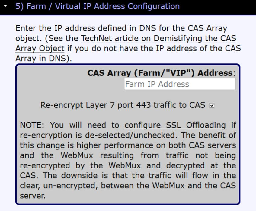
Figure 5 WebMux CAS Array Farm Settings
