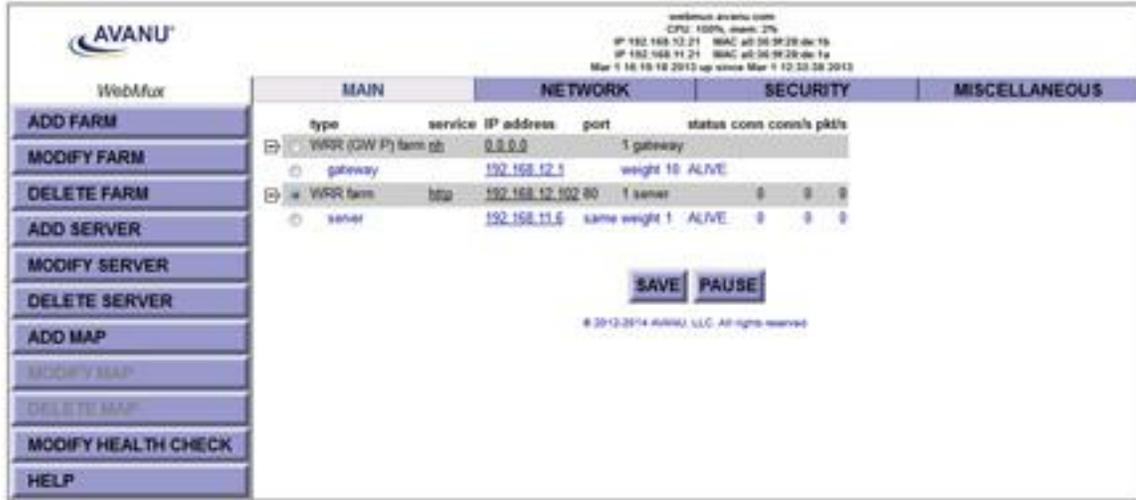
Your original default external gateway will be automatically added to the gateway farm. Click on the gateway farm IP on the grey line above the router IP to add more gateways to the gateway farm.
