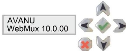
After the unit has fully booted, you will see a scrolling instruction screen. Hold down the Check-Mark button on the WebMux until the LCD displays the first question - "Enter WebMux host name."
