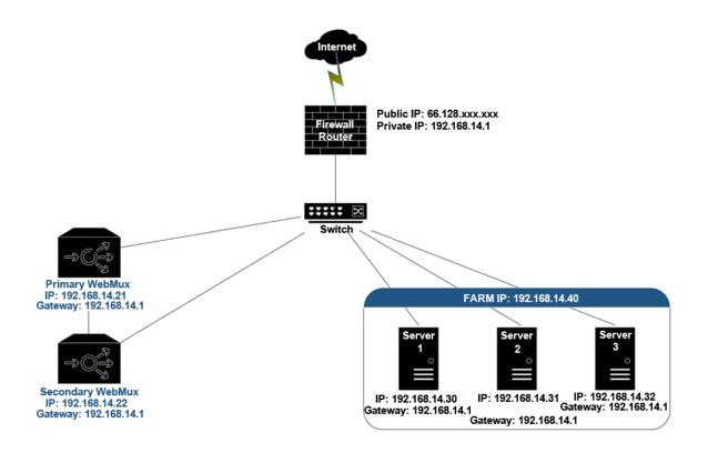
In Single Network Mode, connections being load balanced and going to the real servers will appear to come from the WebMux itself. You will not need to make any changes on your servers since the servers will always reply back to the WebMux when sending back their reply. You will only need to connect the "server LAN" side of the WebMux to the network. Do not connect the "router LAN" side interfaces to your network.
