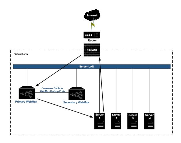
In most situations, incoming traffic is in small requests and return traffic from servers back to clients is large amounts of data (pictures or documents). Using Direct Server Return Mode will allow up to 100 times more traffic to be handled by the WebMux load balancer. The disadvantage for DSR Mode is that the inherent firewall protections of NAT Mode will no longer function. Users must provide their own firewall for incoming and outgoing traffic.
