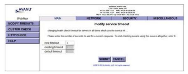
The setting in this page will determine how long or how short the WebMux will wait to be able to verify if the gateway IP is still valid or not. You can disable the checking altogether by setting the timeout value to 0 or you can set the "front network verification" protocol to "none" in the Net work Setup section within this User Manual.
