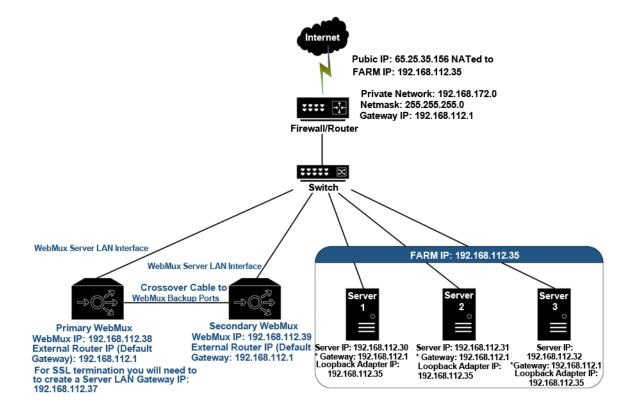
The above diagram is an example about how to configure the WebMux in DSR Mode without changing the IP addresses of the web servers and other servers that already exist on the network. This is another option that can be used if changing the existing network topology of the servers causes problems.
