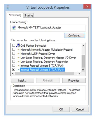
In the "Internet Protocol Version 4 (TCP/IPv4) Properties" screen, enter the FARM IP that the server belongs to and the subnet mask. Do not put anything in the gateway or DNS fields.
