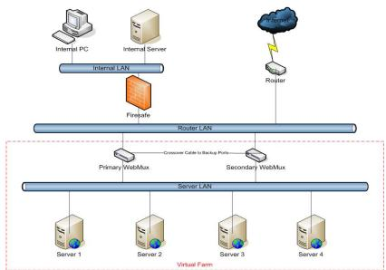
The main purpose of the WebMux is to balance the traffic among multiple web or other servers. The diagram above shows a NAT installation with two WebMux units. In this configuration, one WebMux is serving as the primary, and the other is serving as the secondary, or backup, providing a fault tolerant solution.
