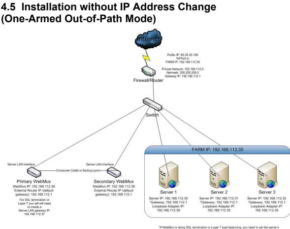
\*If WebMux is doing SSL termination or Layer 7 load balancing, you need to set the server's default gateway IP to the WebMux Server LAN gateway IP: 192-168.112.37
