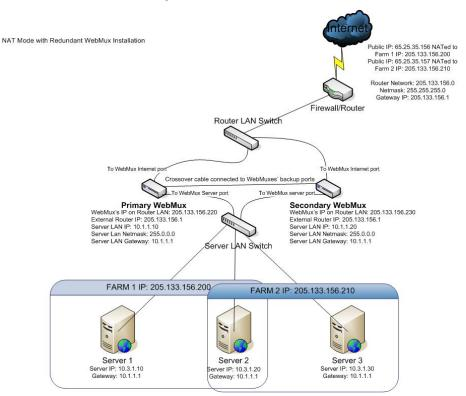
• The installation requires two WebMux units. One will be the primary, and the other the secondary. They connect together with the Ethernet cable that is either cross-over or through a hub or switch. The primary's Backup interface IP address is 192.168.255.253; the secondary's Backup interface IP address is 192.168.255.254. They cannot be changed.
