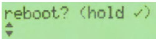
This is the end of initial configuration. Most of the setup or changes require a reboot to take effect. Press and hold the center Check-Mark button to make the WebMux reboot. Use the UP arrow button to return to “Discard Changes” and select “Yes” to exit without change. Press the DOWN arrow or Cross Button to continue to the Factory Reset option (see **Factory Reset** below).
