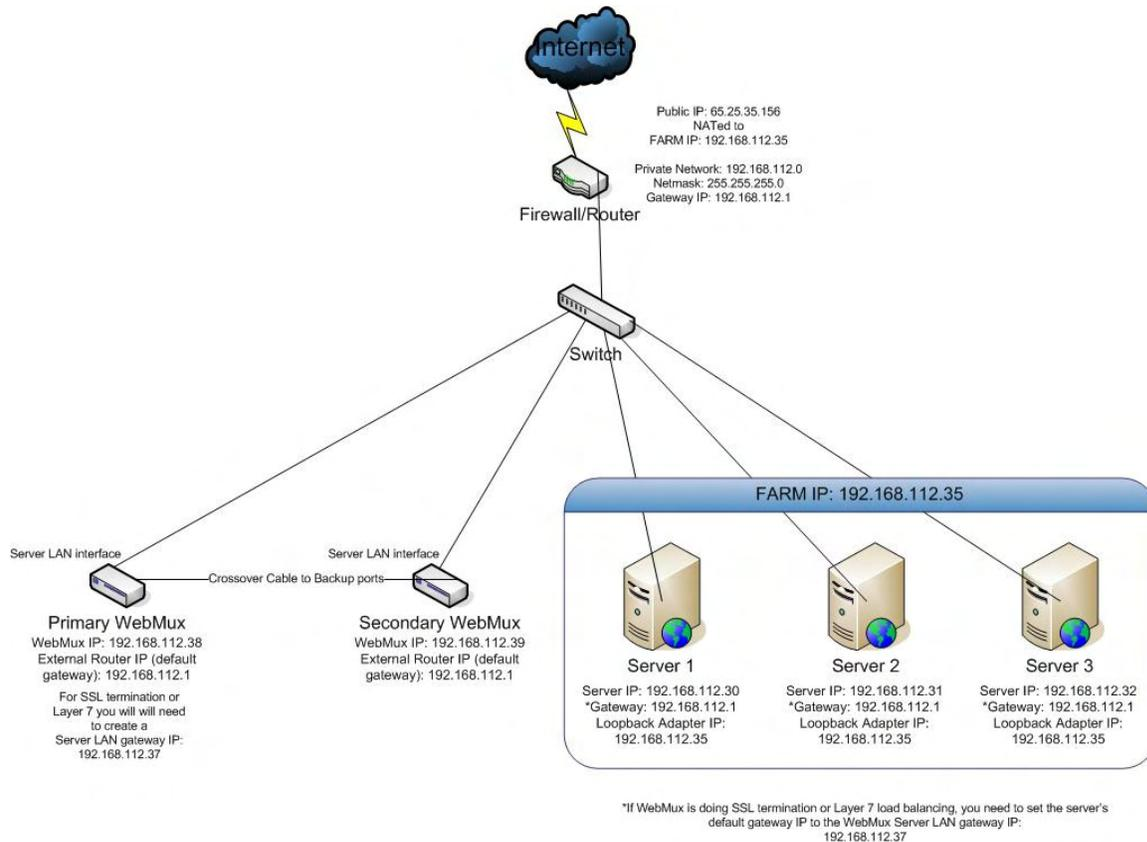
The above diagram is an example about how to configure the WebMux in Out-of-Path mode without changing the IP addresses of the web servers and other servers that already exist on the network. This is particularly helpful when the changing of an existing network of servers causes problems.
