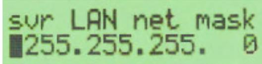
This is the network mask of the Server LAN. For a class A network, it may be 255.0.0.0. For a class C network, it may be 255.255.255.0.
