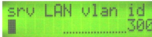
This is the optional VLAN ID tag that will be used for the Router LAN (Internet) interface. You may enter values from 1 – 4067. The cursor position will only go from 0 to 9. To enter a value greater than a single digit, press the left arrow button to move the cursor to the next digit. Enter zero (0) to disable the VLAN ID for the Router LAN (Internet) interface.
