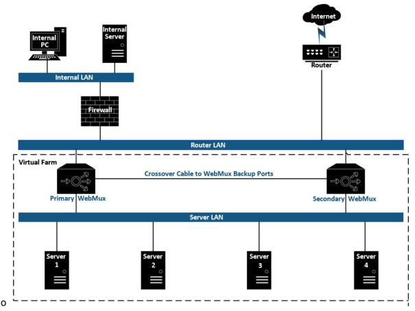
The main purpose of the WebMux is to balance IP traffic amongst multiple web, or other, servers. The diagram above shows a NAT installation with two WebMux units. In this example, one WebMux is serving as the primary, and the other is serving as the secondary, or backup, providing a fault tolerant solution (also called High Avaliability or HA).
