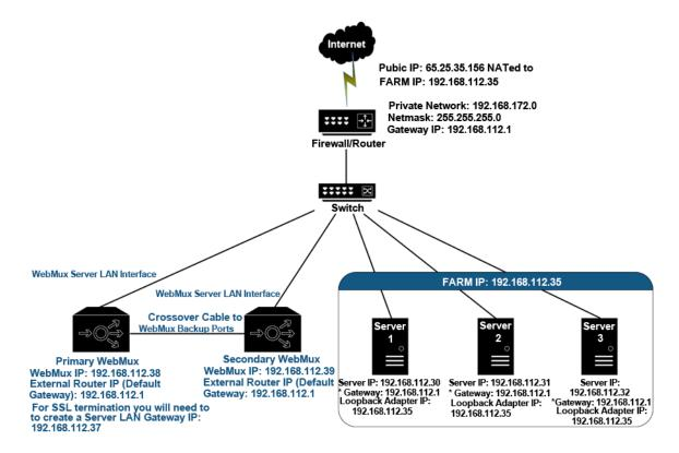
The above diagram is an example about how to configure the WebMux in DSR Mode without changing the IP addresses of the web servers and other servers that already exist on the network. This is another option that can be used if changing the existing network topology of the servers causes problems.
